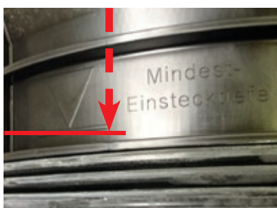
Insert to at least the minimum depth!
