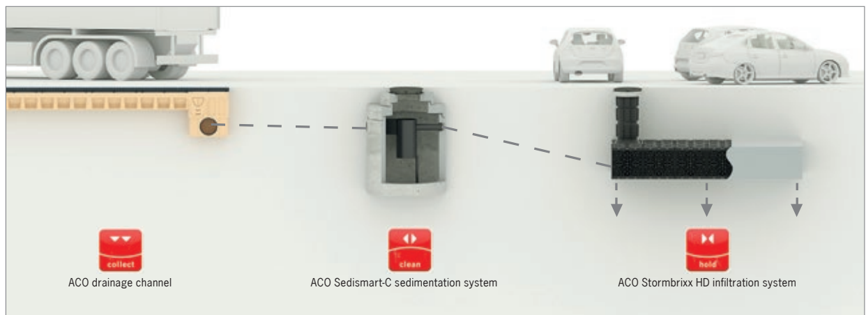
Application example of ACO system chain for rainwater infiltration with ACO Stormbrixx
