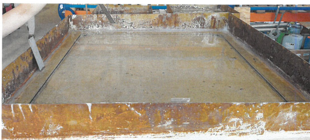
Figure 3: Watertightness test set up – ACO Access Cover PAVING H80 assembly 600x600 D400
