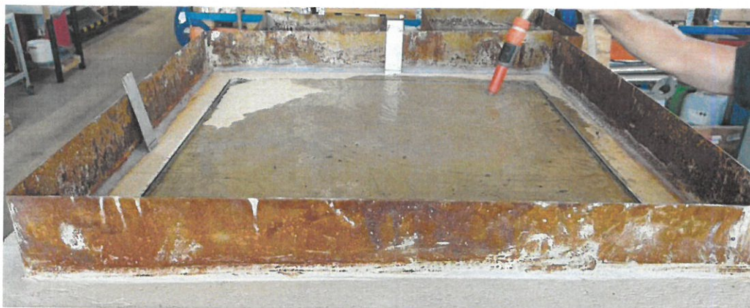
Figure 1: Watertightness test set up – flooding - ACO Access Cover PAVING H80 assembly 600x600 D400
