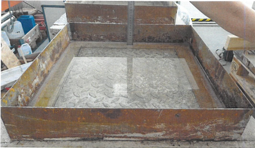
Figure 1: Watertightness test set up - ACO Access Cover SOLID assembly 300x300x60 B125
