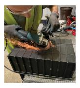
4 Angling the angle grinder, work on the outer perimeter of one of the four segments, do this by rolling the disc around the edge to weaken the segment.
