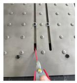
When the slots on the cover are open, you should also spray white lithium grease through these slots onto the top of the PVC below.
