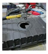
6 For the 3 remaining segments, you can just break these off with a blow from a hammer.
