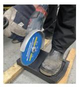
2 Cut the end cap using a disk cutter along the line you marked earlier.
