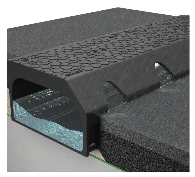
ACO KerbDrain® BridgeDeck is available in both Half Battered and Splayed profiles, each with their own set of problem-solving components ranging from access units to ensure the system can be effectively maintained, as well as outlet connectors and multifunctional end caps.
