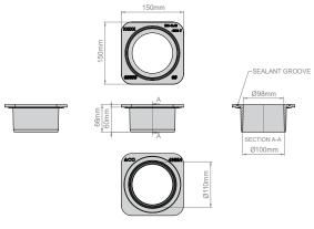
$\emptyset$ 160mm KerbDrain BridgeDeck outlet connector
