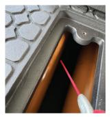
Working on the right-hand access channel facing the road, take your lithium white grease can and spray the PVC pipes located in the access channel through the opening on top of the channel.
