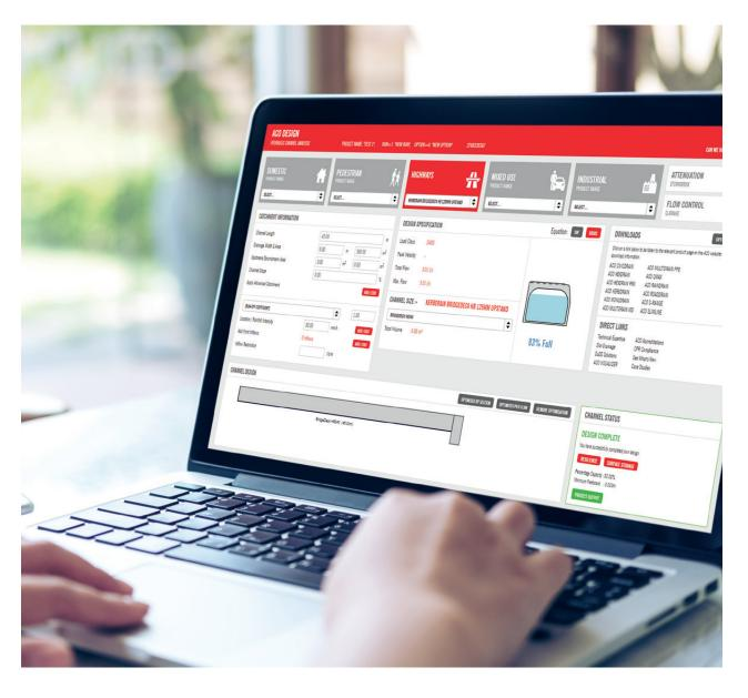
ACO QuAD Hydraulic Design software uses differential equations for spatially varied flow that online alternative solutions cannot accurately match. For example the Manning's equation for steady uniform flow does not work with level channels and is grossly inaccurate on shallow gradients.
