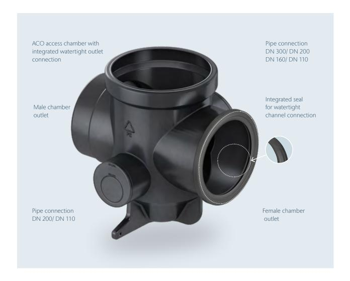
Standard access chamber is ready for 180° connection of the same size of the channel.
