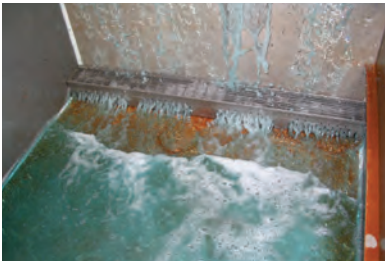
Testing the channel body with mesh grating 30 x 10 mm, free gully with raised coating
