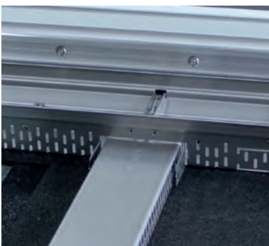
Insertion of the branch channel into the channel. It is recommended using min. 2 branch channels with a length of 50 cm per metre of channel
