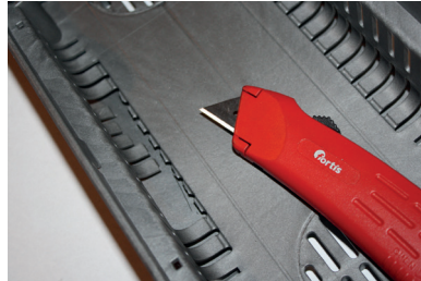
Cut through the ribs from above Press the ribs outwards
