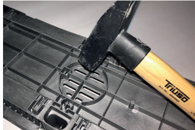
Knock out the area for the insert spigots
