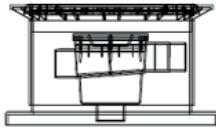
High sliding neck section (with built-in tank filter for house & garden) with walkonable cover
